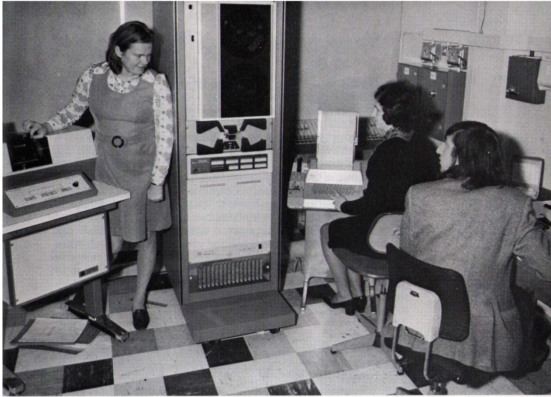
Optronics film scanner and control computer
