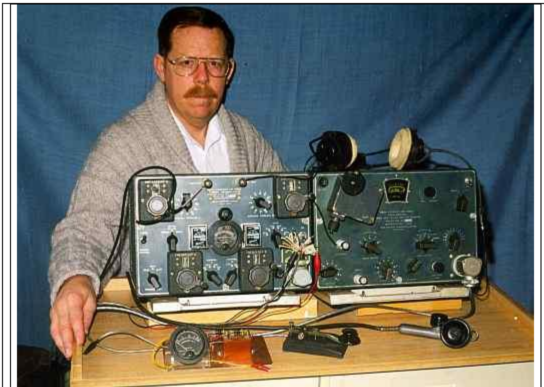
Dave Lawrence, VA3ORP, with a radio station from one of the RCAF Marine Craft. At the left is the AT-1 transmitter. At the right is the AR-6 receiver. The ammeter in the foreground would be used to measure antenna current but it was not part of the original kit.
