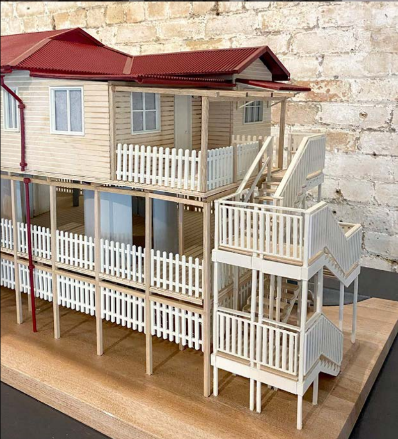
Streetscapes of the Northern Rivers. Illustrations by Rick Shearman. (Below) Exploring house raising and retrofitting designs to get living spaces above future flood levels. Model by Benjamin Brennan.
