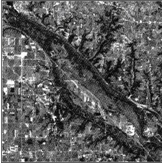
Figure A-2. Example of Nyquist Frequency CN in Band 1 in Landsat 5 MSS Image
