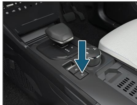
AVH holds the brakes once vehicle speed reaches zero at traffic lights or a junction, thus avoids unintended vehicle rolling. Once activated through AVH switch Automatic Vehicle Hold maintains brake force even after you release the Brake Pedal. You can then release the brake pedal and remain stopped, even on a hill.
