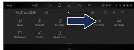
The system also displays the Park assist screen when the reverse gear is engaged. It provides audio and visual information through the vehicles infotainment system / Buzzer.
