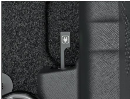
6. Open the protective cap on Charging Inlet.
