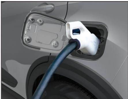
10. Charging Gun will be locked after switching on the DC charging station.
