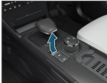
2. Pull the 'Charging-inlet Flap Open Lever' to open the charging inlet flap.
