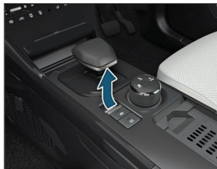
EPB switch is located behind the Mono shift knob EPB is applied by pulling up the EPB switch and can be released by pushing down the EPB switch which needs the vehicle to be at ignition ON condition. Always ensure parking brake is released and parking brake warning lamp is OFF before start of the drive. Park brake warning lamp in cluster at vehicle running condition indicates failure in brake system needs to be checked with TATA MOTORS EV Authorised Service Centre and vehicle
