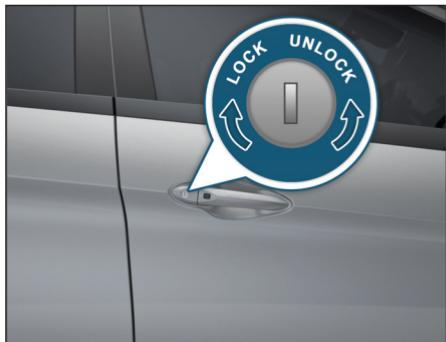
Driver door can be locked or unlocked from outside using the key blade.
