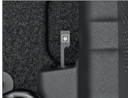
3. Open the protective cap on Charging Inlet (AC side).
