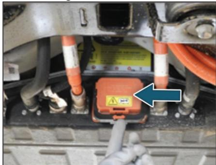
age components he should remove the HV MSD connector.
