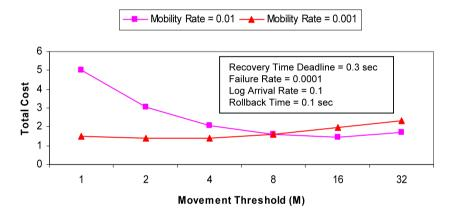
Fig. 9 Determining optimal movement threshold that minimizes recovery cost per failure
