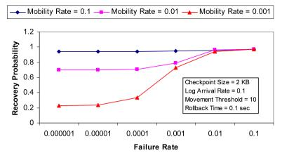
Fig. 6 Recovery probability vs. failure rate
