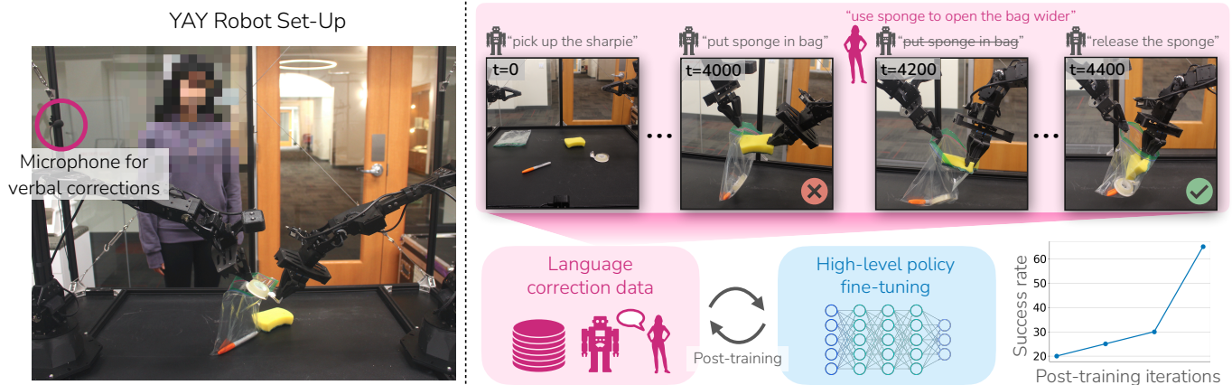
Fig. 1: Our approach enables robots to leverage verbal corrections to improve performance on complex long-horizon tasks like packing a ziploc bag and preparing trail-mix. It can incorporate verbal corrections in real-time (top) and for continuous improvement (bottom).
