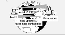
The base transaction generated by a tentative transaction may fail or it may produce different results. The base transaction has an *acceptance criterion*: a test the resulting outputs must pass for the slightly different base transaction results to be acceptable. To give some sample acceptance criteria:
