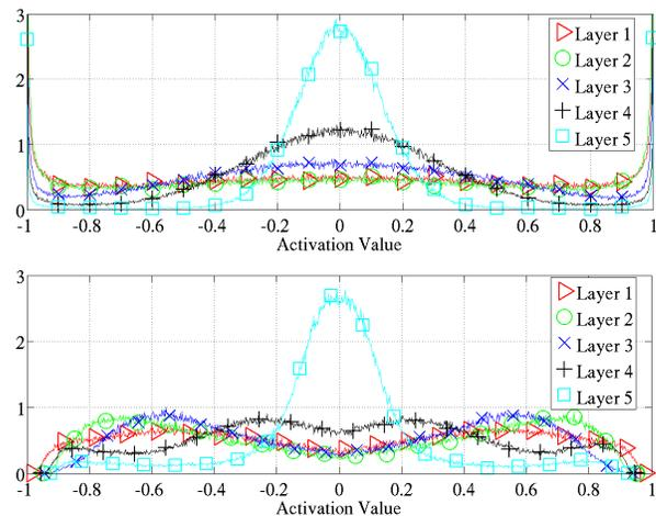
Figure 4: *Activation values normalized histogram at the end of learning, averaged across units of the same layer and across 300 test examples. Top*: activation function is hyperbolic tangent, we see important saturation of the lower layers. *Bottom*: activation function is softsign, we see many activation values around (-0.6,-0.8) and (0.6,0.8) where the units do not saturate but are non-linear.
