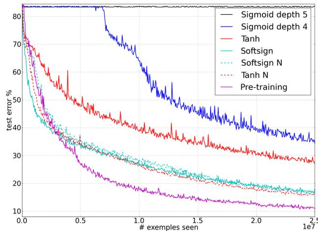
Figure 11: Test error during online training on the **Shapenet-3**  $\times$  2 dataset, for various activation functions and initialization schemes (ordered from top to bottom in decreasing final error). *N* after the activation function name indicates the use of normalized initialization.
