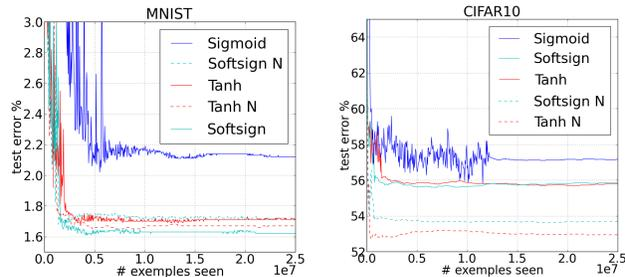
Figure 12: Test error curves during training on **MNIST** and **CIFAR10**, for various activation functions and initialization schemes (ordered from top to bottom in decreasing final error). *N* after the activation function name indicates the use of normalized initialization.
