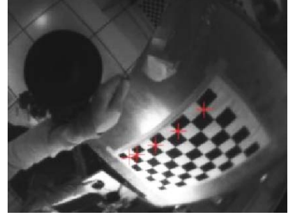
Fig. 6. Estimation of the focal length from line image points
