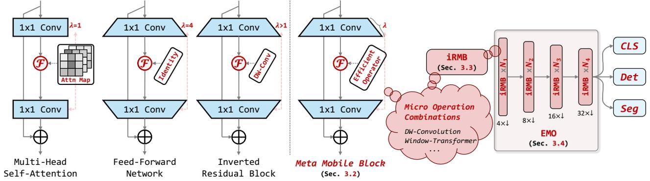
Figure 2: **Left:** Abstracted unified **Meta-Mobile Block** from *Multi-Head Self-Attention / Feed-Forward Network* [66] and *Inverted Residual Block* [54] (c.f. Sec 2.2). The inductive block can be deduced into specific modules using different *expansion ratio*  $\lambda$  and *efficient operator*  $\mathcal{F}$ . **Right:** ResNet-like *EMO* composed of only deduced *iRMB* (c.f. Sec 2.3).
