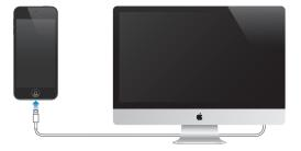
*Important:* The iPod touch battery may drain instead of charge if iPod touch is connected to a computer that's turned off or is in sleep or standby mode.
