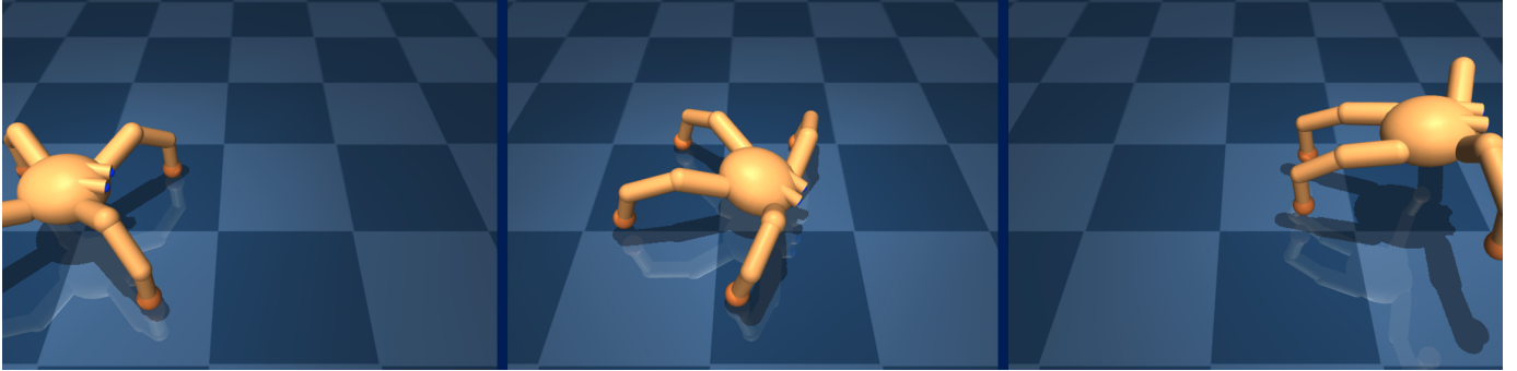
(b) Differentiable tube-based MPC. The adaptation enables the quadruped to successfully reach the target despite large disturbances.
