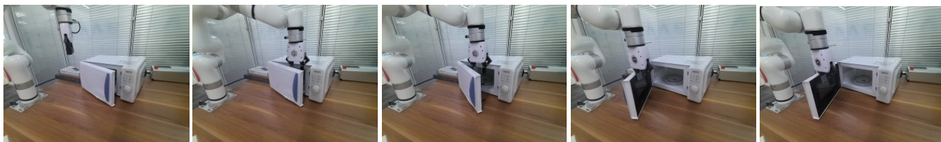
(a) Nudge the microwave's door open
