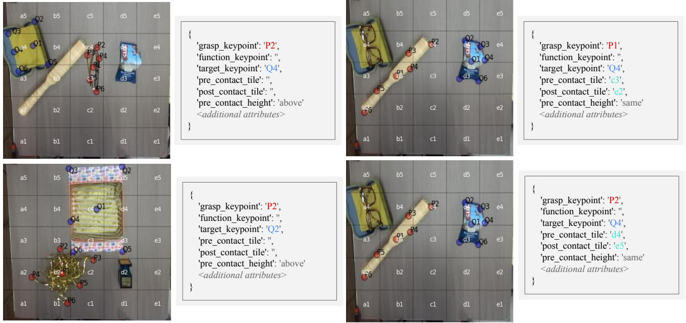
Fig. 8: Qualitative results of ablation studies. Without the keypoint description or chain-of-thought prompting, the model can make mistakes in keypoint prediction (left column) and waypoint prediction (right column).
