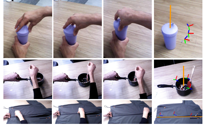
Fig. 3. Human demonstrations as screw actions. Three frames of a human demonstration for three bimanual tasks (top row: opening a bottle, m = \text{revolute} , middle row: stirring a pot, m = \text{revolute3D} , bottom row: opening a zipper, m = \text{prismatic} ) and the perceived screw axis explaining the motion (fourth column, orange indicates the axis line). Our screw action representation facilitates the interpretation of noisy hand trajectory observations in a bimanual interaction as evidence of a simple 1-DoF constraint between both hands
