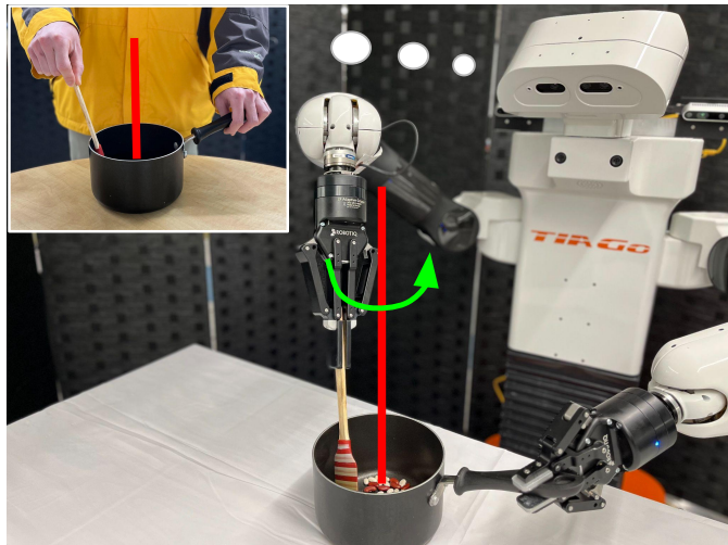
Fig. 1. Bimanual manipulation tasks can be represented by a screw axis (red line) constraining and synchronizing the motion of both hands. SCREWMIMIC maps a single human demonstration into a screw axis, improves it with an iterative interactive exploration procedure, and learns to predict it for new object instances and poses, enabling their manipulation.
