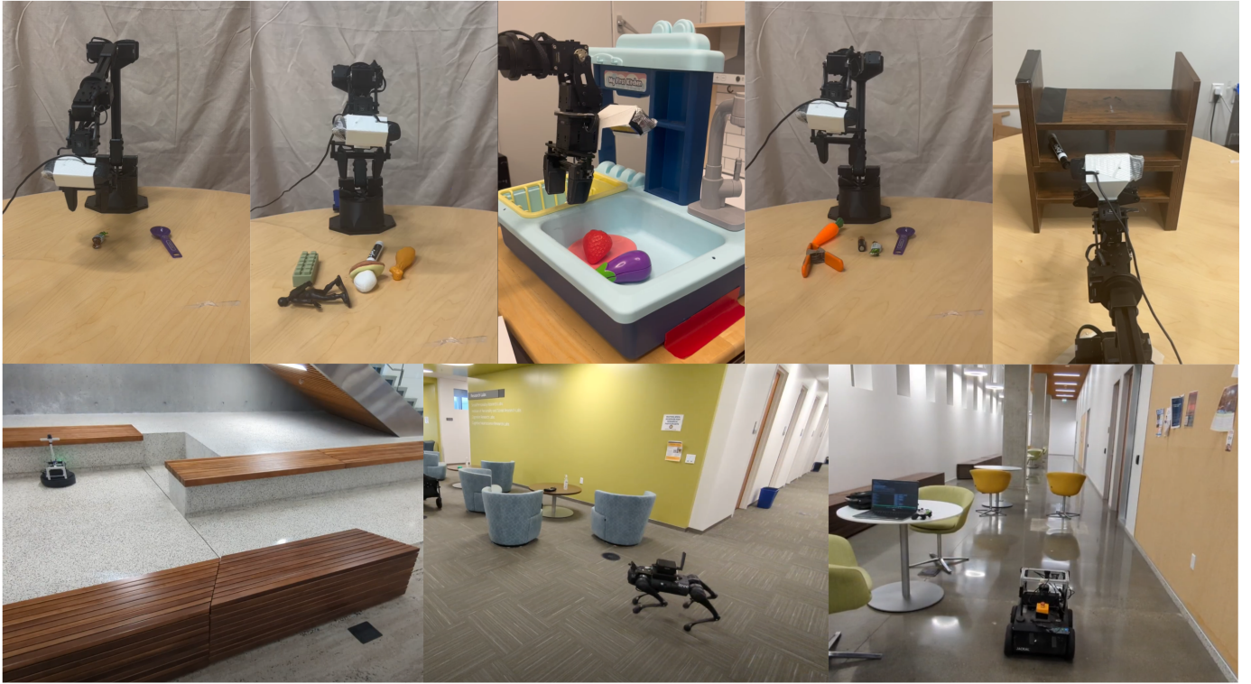
Fig. 9: Navigation and Manipulation Tasks. We evaluate our policy’s manipulation performance on the two-object grasp, cluttered grasp, toy kitchen, cluttered grasp novel, and shelf manipulation tasks (from left to right). To evaluate our policy’s navigation performance, we run our policies on the LoCoBot, Unitree Go-1 and ClearPath Jackal (from left to right).
