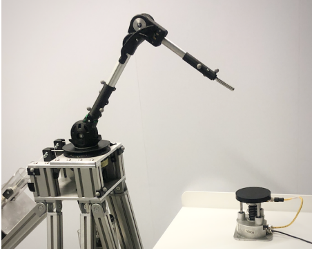
Fig. 4: Experimental setup for the collision force measurements. A Pilz PRMS is mounted to a table onto which the end effector of the robot is colliding.
