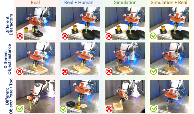
Fig. 9: Domain Composition Comparison. By composing policies trained in simulation, human, and real data, our approach can generalize across multiple distractors (first row), with varying object and tool poses (second row), and across new object and tool instances (third row).
