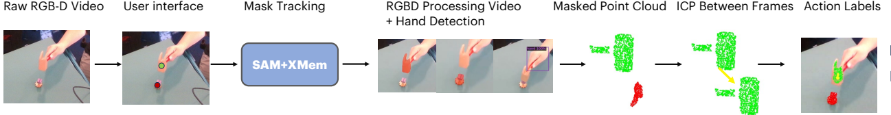
Fig. 5: Dataset Processing Pipeline. We show the human demonstration video collected in the wild from uncalibrated RGB-D cameras can be converted into a labeled trajectory (relative tool poses). The same pipeline applies to evaluating policy in the real world.
