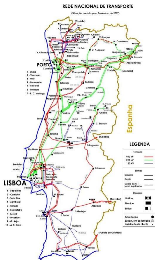
Figure 52 - Map of the National Electricity Transmission Network in 2017 [Source: REN, 'Indicative interconnection capacities for commercial purposes in 2017']
