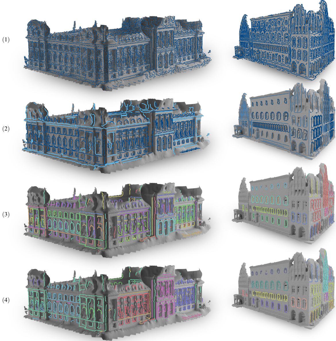
Figure 3: Scan of a museum (left) and a townhall (right), with (1) the initial dense feature network generated with [YBS05]. (2) shows the completed FCN. (3) depicts the connected components. (4) shows the feature curve groups that fall into the same template. Dark blue curves indicate the reoccurring templates, while strong (non-reoccurring) curves are visualized in light blue.
