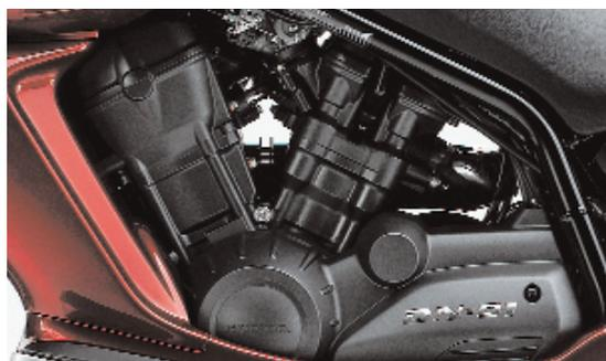
**Left:** The DN-01's 52° V-twin has its roots in the NT650 Hawk of 1968. The current Euro-only XL700V Transalp has it too, but it's retuned and uses a conventional gearbox. The DN-01 is tuned for low- and mid-range power.
