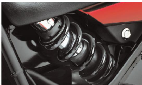
**Above:** The DN-01's single shock is made by Showa and controls the single-sided Pro Arm swingarm without the aid of rising rate linkage. The shock offers seven steps of preload adjustability but does not have any compression or rebound damping adjusters.
