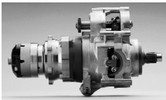
**Above:** The heart of the DN-01 is not its engine, but rather its Human Friendly Transmission, a maintenance-free (says Honda) fluid-power unit that provides the DN-01 with seamless shifting performance and infinitely variable gear ratios when used in the Drive or Sport modes. But it can also be shifted manually via a control on the left handlebar.
