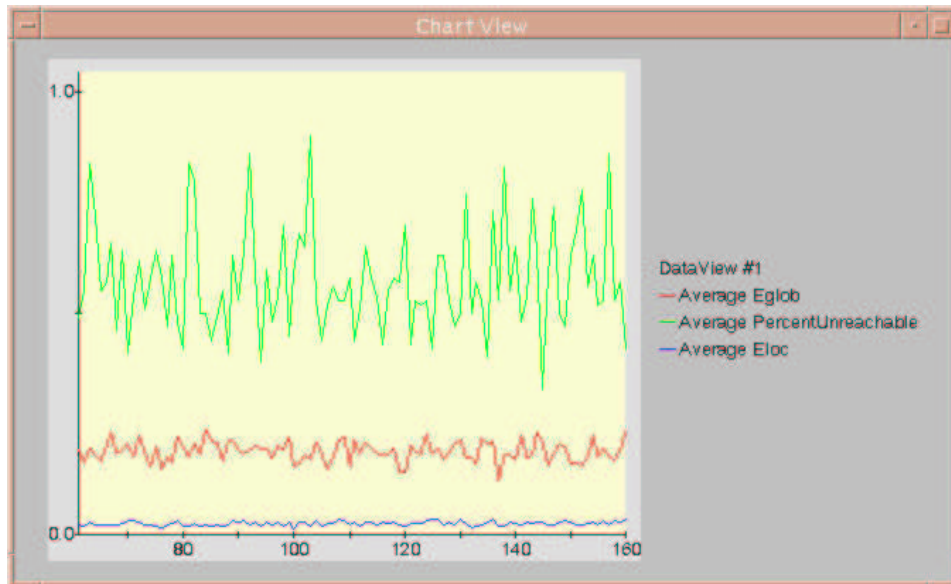
Figure 6: Metrics plotted versus time (rounds). Every peer has 5 friends and N=100 . Peers can fail independently with 0.4 probability per round. Keep-alive hop count=4.
