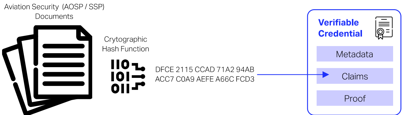
Figure 12 – Illustration of including cryptographic hashes of aviation security document in a VC
