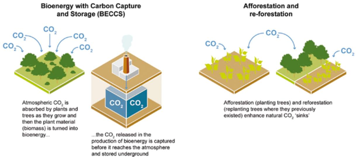
**FAQ 4.2, Figure 1 | Carbon dioxide removal (CDR) refers to the process of removing CO<sub>2</sub> from the atmosphere.** There are a number of CDR techniques, each with different potential for achieving 'negative emissions', as well as different associated costs and side effects.
