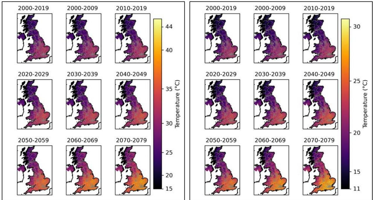
**Figure 5.6** Decadal ensemble means in the annual daily temperature maxima (left panels) and in the summer average daily maximum temperatures (right panels) using 120 'years' of CPM data for each decade.
