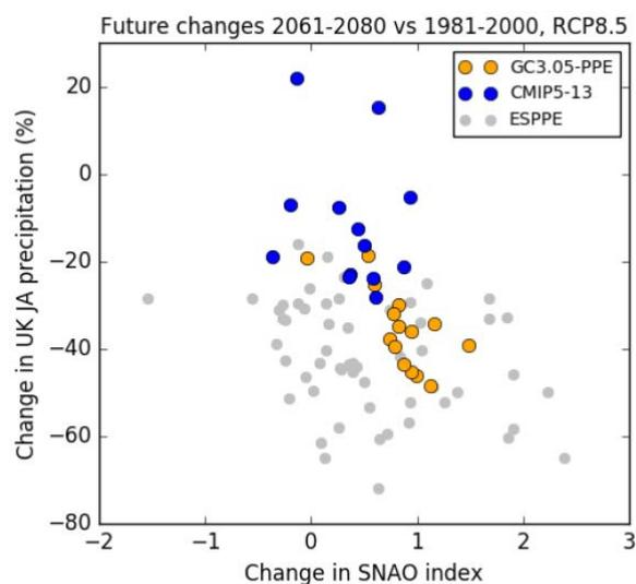
**Figure 5.3** Relationship between projected changes in the SNAO and UK high summer rainfall from the CMIP5-13 ensemble with the standard RCP8.5 concentrations (blue) and HadGEM3 GC3.05 ensemble with RCP8.5 emissions (orange). The grey dots refer to a larger ensemble of from a lower-resolution Earth System model using RCP8.5 emissions. Reproduced from UKCP18 Land Report, Murphy et al. (2018)<sup>5</sup>.
