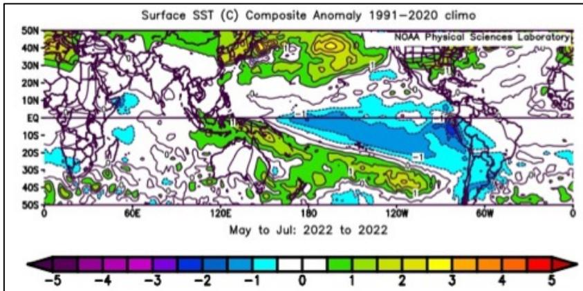
**Figure 3.2** Sea surface temperatures anomalies ( $^{\circ}\text{C}$ ) for the 3 months (May – July 2022) preceding the July heatwave showing colder than normal water in the East Pacific, typical of La Nina conditions. (Source: NOAA)
