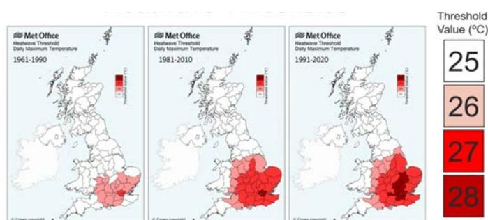
**Figure 2.1** Heatwave threshold temperatures (°C) across the UK as updated in January 2022 and based on the most recent 30-year climatology. (Source: Met Office)
