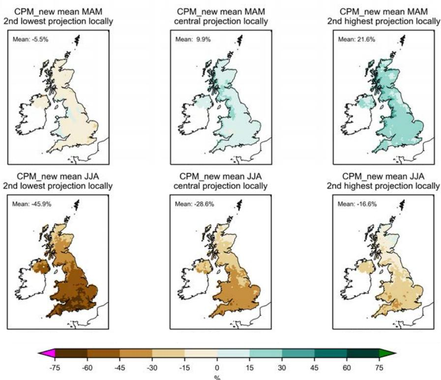
**Figure 5.16** Projected future changes in spring (upper panels) and summer (lower panels) mean precipitation (%) for 2061-2080 from the 1981-2000 baseline from the UK CPM ensemble for the RCP8.5 emissions scenario. Changes are shown for 2nd lowest (left), central (centre) and 2nd highest (right) member locally. (Source: Met Office)
