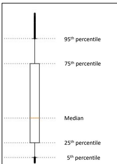
**Figure 5.8** Schematic of how the probabilities are presented.
